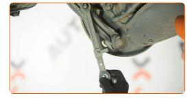
Clean the fastener of the ABS sensor bracket. Use a wire brush. Use WD-40 spray.
