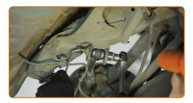
Remove the support from under the arm.
