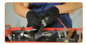
Tighten the bracket fastening to the arm. Use Torx T20. Use a ratchet wrench.
