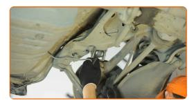
Tighten the fastener connecting the suspension arm to the rear knuckle. Use a combination spanner #17. Use a torque wrench. Tighten it to 40 Nm torque.
