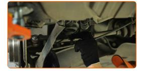
18 Install the rear fastener of the control arm.
