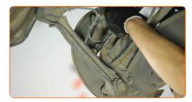
Connect the ABS sensor wiring.
