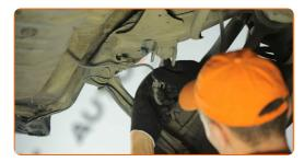
Remove the arm. Use a ball joint puller.
