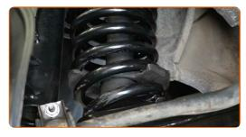
Remove the coil spring compressor.
