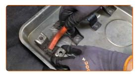
15 Install the anti-roll bar.
