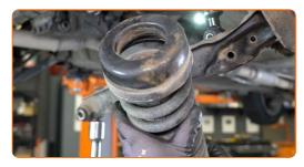
Clean the coil spring mounting seats. Use a wire brush. Use all-purpose cleaning spray.
