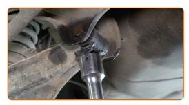
Unscrew the fastener connecting the control arm to the subframe. Use a combination spanner #19. Use a drive socket #19. Use a ratchet wrench.
