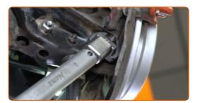
Tighten the fastener connecting the control arm to the subframe. Use a combination spanner #19. Use a drive socket #19. Use a torque wrench. Tighten it to 70 Nm torque.
