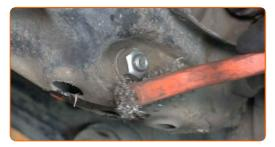
Support the rear control arm. Use a hydraulic transmission jack.
