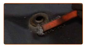
Clean the control arm fasteners. Use a wire brush. Use WD-40 spray.
