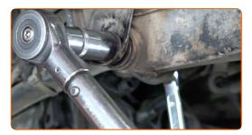
Tighten the lower fastener of the shock absorber. Use a combination spanner #17. Use a drive socket #17. Use a torque wrench. Tighten it to 55 Nm torque.
