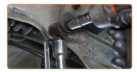
Remove the fastening bolt. Use a pin punch. Use a hammer.
