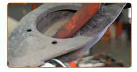
Clean the suspension arm mounting seats. Use a wire brush. Use all-purpose cleaning spray.
