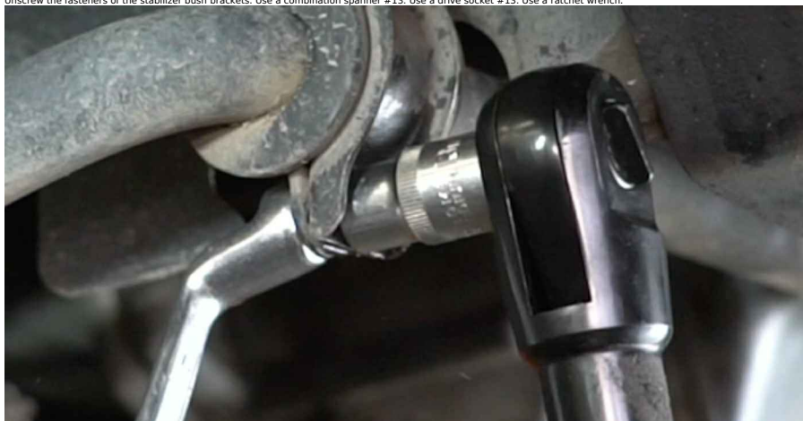
16 Remove the fastening bolts.
