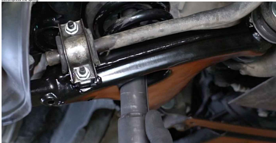
32 Remove the coil spring compressor.
