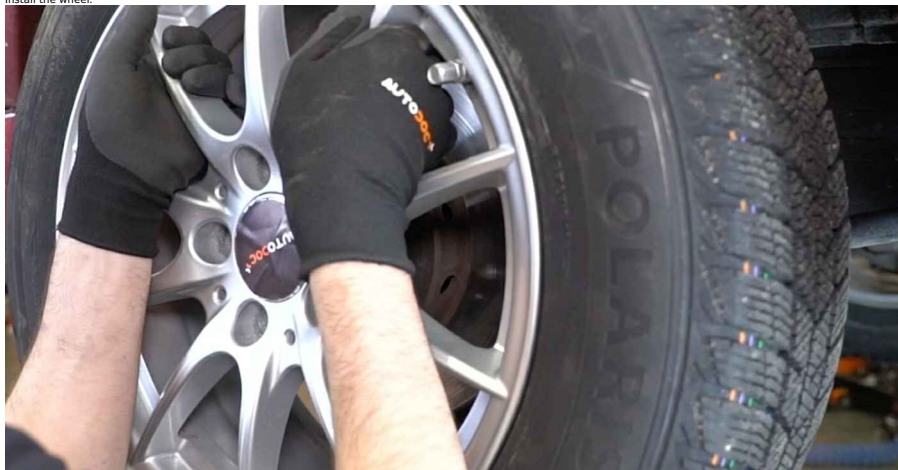
Replacement: coil springs - MERCEDES-BENZ E-Class Coupe (C124). AUTODOC recommends: • To avoid injury, hold up the wheel when screwing in the fastening bolts.
