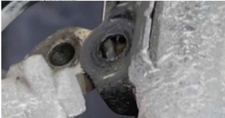
14 Clean the fasteners of the stabilizer bush brackets. Use a wire brush. Use WD-40 spray.
