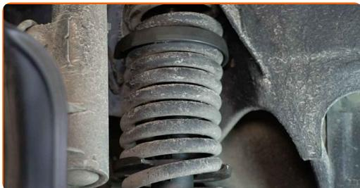
Replacement: suspension strut – MERCEDES-BENZ E-Class Coupe (C124).
