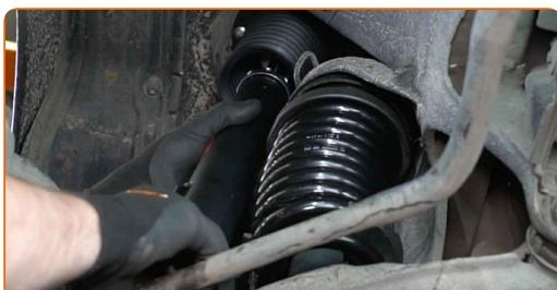
**Replacement: suspension strut – MERCEDES-BENZ E-Class Coupe (C124). Tip from AUTODOC experts:**
