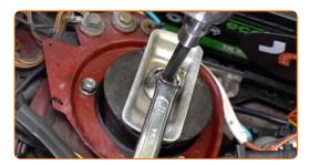
Replacement: suspension strut – MERCEDES-BENZ E-Class Coupe (C124). Tip:
