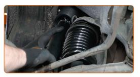
Replacement: suspension strut – MERCEDES-BENZ E-Class Coupe (C124). Tip from AUTODOC experts:
