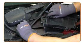
Press on the cabin filter retainer to release it.
