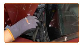
Unscrew the fasteners of the drain. Use a Phillips screwdriver.
