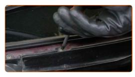
6 Remove the side part of the drain.
