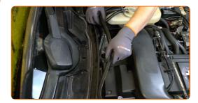
Remove the central element that holds the seal of the windscreen wiper scuttle tray.
