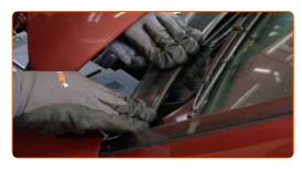
Install the central element that holds the seal of the windscreen wiper scuttle tray.
