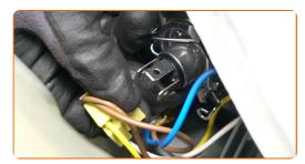
Pull aside the retainer of the low and high beam bulb.
