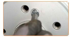
Tighten the brake disc fasteners. Use HEX No.H5. Use a torque wrench. Tighten it to 10 Nm torque.
