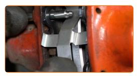
Install the brake pad guide pins. Use a pin punch. Use a hammer.
