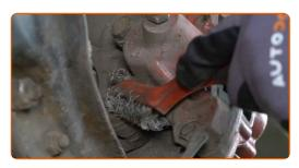
Unscrew the brake caliper fasteners. Use a combination spanner #17.
