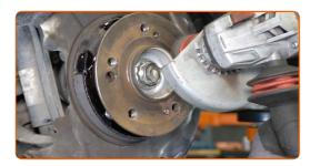
Treat the contacting surface. Use ceramic grease.
