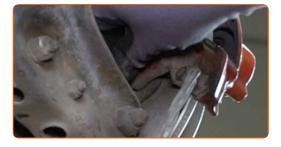
Tighten the brake caliper fasteners. Use a drive socket #17. Use a torque wrench. Tighten it to 65 Nm torque.
