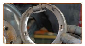
Clean the mounting seats of the parking brake shoes. Use a wire brush. Use all-purpose cleaning spray.
