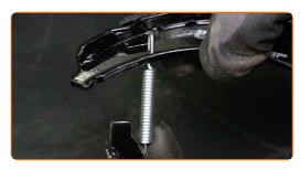
Install the parking brake adjuster.
