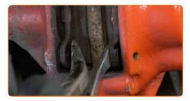
Remove the brake pads.
