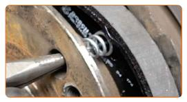
Install the lower return spring. Use a flat screwdriver.
