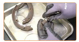
Clean the parking brake adjuster. Use a wire brush. Use all-purpose cleaning spray.
