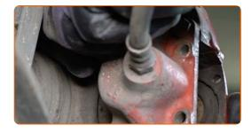
16 Remove the brake caliper.
