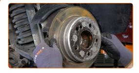
Remove the lower brake shoe return spring. Use a flat screwdriver.
