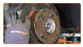
Remove the parking brake adjuster.
