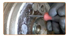
Remove the brake disc.
