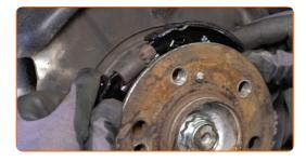
Install the hold-down springs of the parking brake shoes. Use long nose pliers.
