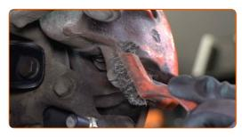
Unscrew the brake caliper fasteners. Use a combination spanner #15. Use a drive socket #13. Use a ratchet wrench.
