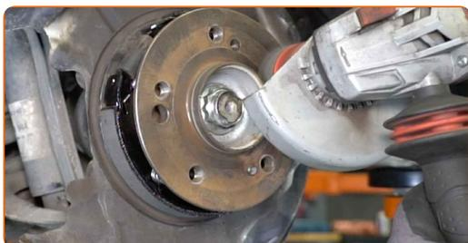
**23** Treat the contacting surface. Use ceramic grease.
