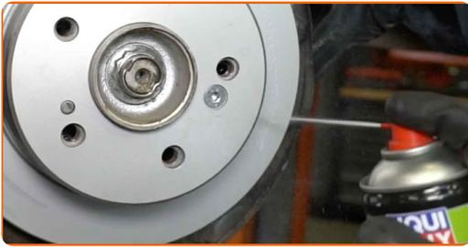
**35** Treat the surface where the brake disc contacts the wheel rim. Use ceramic grease.
