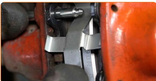
**33** Install the brake pad guide pins. Use a pin punch. Use a hammer.
