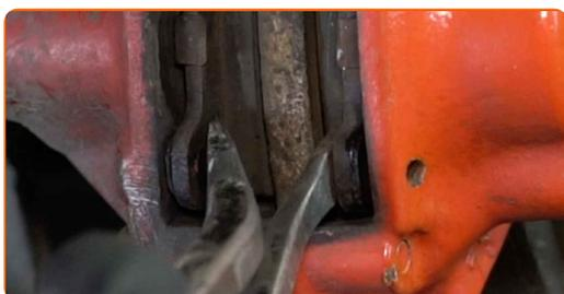
**12** Remove the brake pads.
