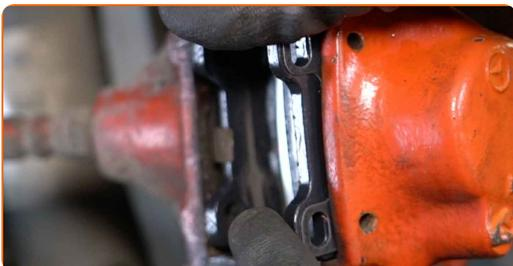
**32** Install the retaining spring of the brake pads.
