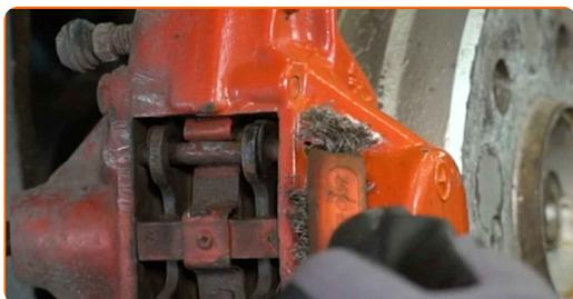
**9** Remove the brake pad guide pins. Use a pin punch. Use a hammer.
