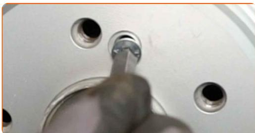
**26** Tighten the brake disc fasteners. Use HEX No.H5. Use a torque wrench. Tighten it to 10 Nm torque.
