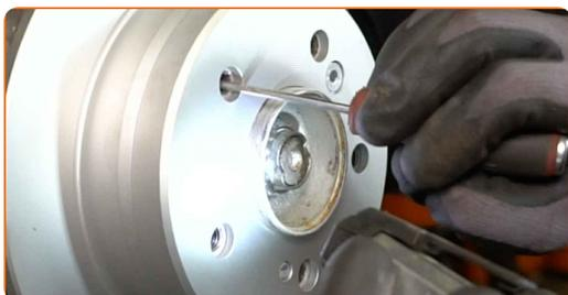
**28** Install the brake caliper and fasten it.
