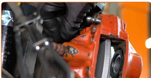
**44** Tighten the brake caliper fasteners. Use a drive socket #17. Use a torque wrench. Tighten it to 65 Nm torque.
