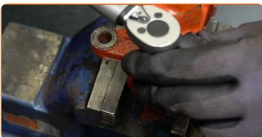
**39** Tighten the brake bleeder screw.
