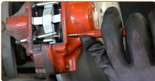
**10** Remove the retaining spring of the brake pads.
