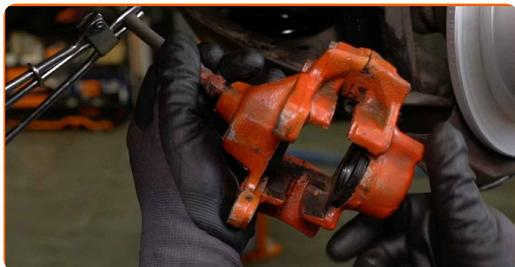
**42** Install the brake caliper and fasten it.
