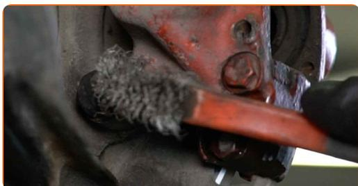
**17** Unscrew the brake caliper fasteners. Use a drive socket #17. Use a ratchet wrench.
