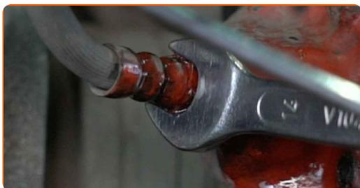
**16** Clean the brake caliper fasteners. Use a wire brush. Use WD-40 spray.
