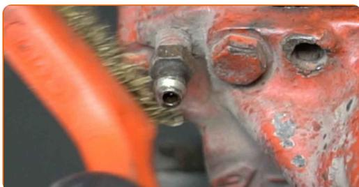
**22** Undo the brake bleeder screw. Use a drive socket #9. Use a ratchet wrench.
