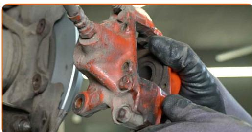
**20** Unscrew the brake hose from the brake caliper.
