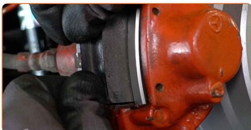
**13** Clamp the brake hose off using a brake hose clamp.
