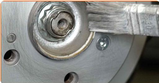
**57** Clean the brake disk surface. Use a brake cleaner.
