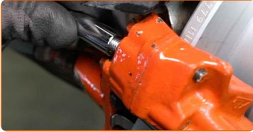
**55** Attach the brake caliper bleed screw cap.
