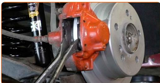
**12** Remove the brake pads.
