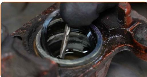
**30** Clean the mounting seats of the pistons and related components. Use a wire brush. Use a nylon cleaning brush. Use all-purpose cleaning spray.
