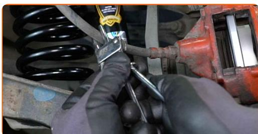
**14** Clean the mounting seat of the brake hose on the brake caliper. Use a wire brush. Use WD-40 spray.
