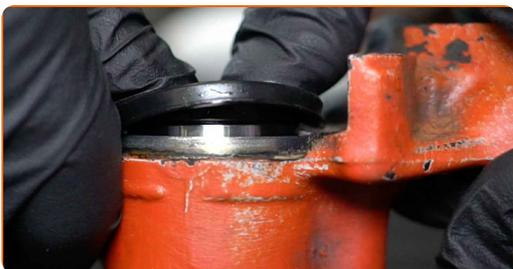
**34** Install dust boot retaining rings.
