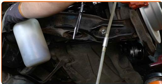
**50** Remove the brake hose clamp.
