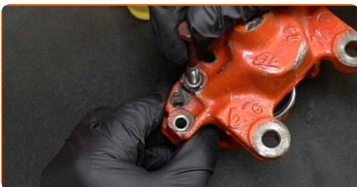
**38** Tighten the fasteners connecting the two parts of the caliper. Use a drive socket #14. Use a torque wrench. Tighten it to 35 Nm torque.
