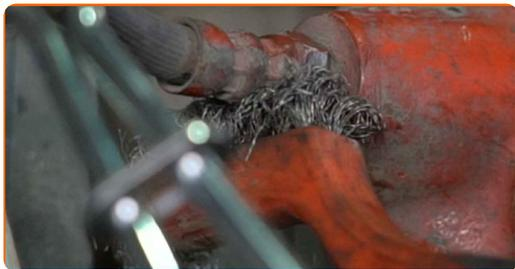
**15** Loosen the brake hose fastener. Use a combination spanner #14.
