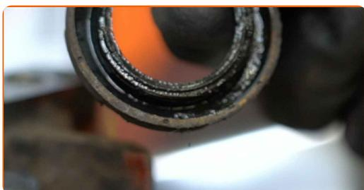
**28** Remove the brake caliper pistons. Use water pump pliers.
