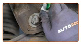
Unscrew the front fastener of the control arm. Use a combination spanner #22. Use a drive socket #22. Use a ratchet wrench.
