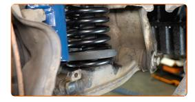
Remove the coil spring compressor.
