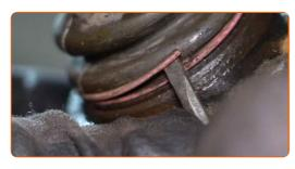
Remove the ball joint boot. Use a flat screwdriver.
