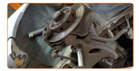
Install the coil spring compressor on the coil spring.
