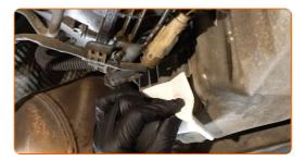
Screw in the new drainage plug and tighten it. Use a drive socket #13. Use a torque wrench. Tighten it to 30 Nm torque.
