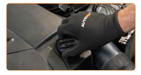
33 Tighten the oil filler cap.
