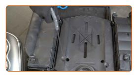
Unscrew the fasteners of the air filter covers. Use Torx T20. Use a ratchet wrench.
