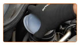
17 Install the air filter housing.
