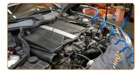
Remove the air filter housing.
