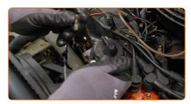
Remove the thermostat together with the housing.
