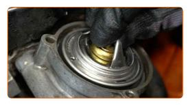
18 Install the thermostat housing.
