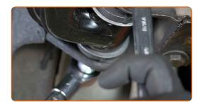
Tighten the front fastener of the arm. Use a combination spanner #22. Use a drive socket #22. Use a torque wrench. Tighten it to 120 Nm torque.
