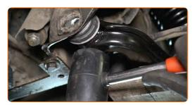
Install the fastening bolts. Use a rubber mallet.
