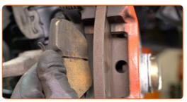
Replacement: brake pads – MERCEDES-BENZ E-Class Convertible (A124). Tip from AUTODOC:
