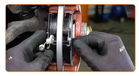
20 Install the brake caliper and fasten it.
