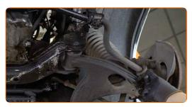
Install the stabilizer bush brackets. Use water pump pliers.
