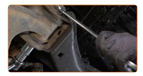
Unscrew the rear fastener of the control arm. Use a combination spanner #22. Use a drive socket #22. Use a ratchet wrench.
