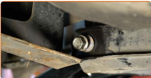
**17** Screw the fastener connecting the control arm to the subframe.
