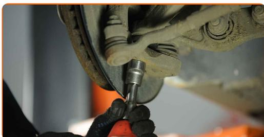
**8** Disconnect the ball joint from the steering knuckle. Use a ball joint puller.
