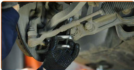
**9** Clean the fasteners connecting the control arm to the subframe. Use a wire brush. Use WD-40 spray.
