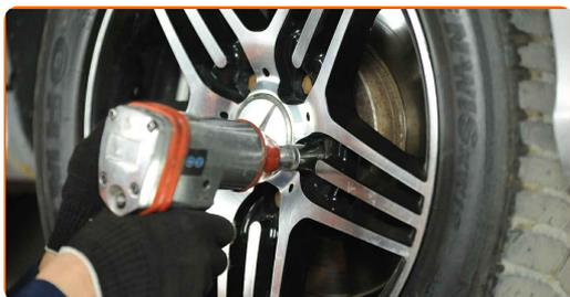
**26** Lower the car and working in a cross order, tighten the wheel bolts. Use wheel impact socket #17. Use a torque wrench. Tighten it to 120 nm torque.
