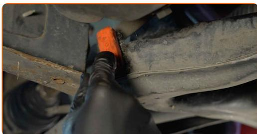
**10** Unscrew the arm fastening from the subframe. Use a combination spanner #21. Use a drive socket #E18. Use a ratchet wrench.
