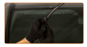
Remove the blade from the wiper arm.
