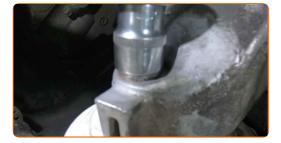
Tighten the upper fastener of the engine mount. Use a drive socket #16. Use a torque wrench. Tighten it to 50 Nm torque.
