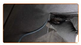
Screw in the fasteners of the side trim panel. Use a Phillips screwdriver.
