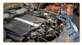
Remove the air filter housing.
