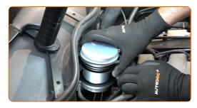
Lock the mass air flow sensor retaining clips.
