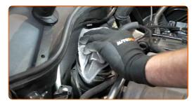
Clean the mounting seat of the mass air flow sensor.
