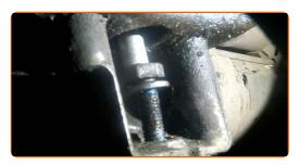
Unscrew the lower fastener of the engine mount. Use a drive socket #13. Use a ratchet wrench.
