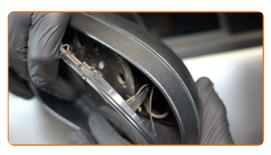
Carefully release the mirror glass from its attachment.
