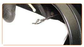
Release the mirror glass retainer clip. Use a flat screwdriver.
