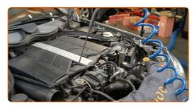
Remove the air filter housing.
