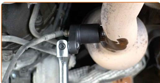
**11** Remove the oxygen sensor.
