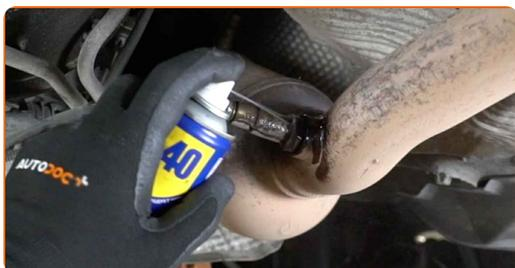
**10** Unscrew the oxygen sensor fastener. Use a 22-mm oxygen sensor socket. Use a ratchet wrench.
