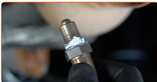
**14** Install the new oxygen sensor.
