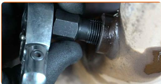
**13** Treat the oxygen sensor. Use high-temperature ceramic grease.
