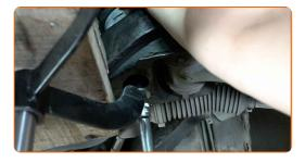
Remove the support from under the engine.
