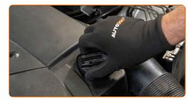
Tighten the oil filler cap.
