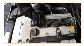
Plug in the ignition coil connector.
