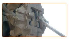
Remove the brake pads.
