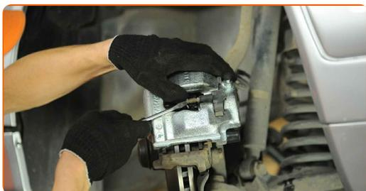
**34** Install the brake caliper retaining spring. Use a flat screwdriver.
