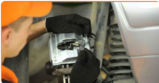
**33** Connect the brake pad wear sensor plug. Use a flat screwdriver.
