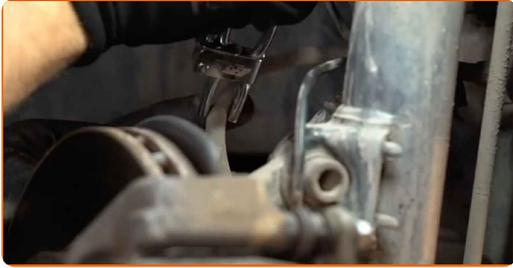
**18** Unscrew the brake hose from the brake caliper. Use a flare nut spanner #14.
