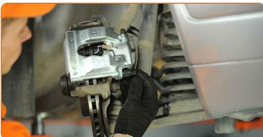
**32** Connect the brake pads wear sensor. Use Torx T30. Use a ratchet wrench.
