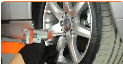
**45** Lower the car and working in a cross order, tighten the wheel bolts. Use wheel impact socket #17. Use a torque wrench. Tighten it to 110 nm torque.
