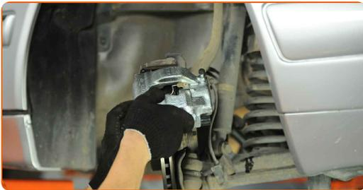
**27** Clean the brake caliper guide pins.
