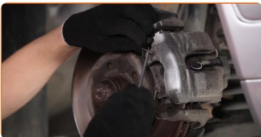
**8** Disconnect the brake pad wear sensor plug. Use a flat screwdriver.
