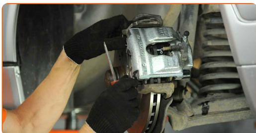
**35** Connect the brake bleeder kit to the brake bleeder screw.
