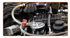
Attach the pipe to the fuel filter.
