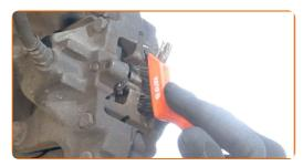
Remove the brake pad retaining pin. Use a pin punch. Use a hammer.
