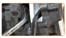
Treat the brake pads in the area where their surface comes into contact with the brake caliper bracket. Use antisqueal paste.
