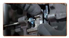
Install the brake pad retaining pin. Use a pin punch. Use a hammer.
