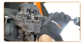
Remove the retaining spring of the brake pads.
