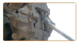
11 Remove the brake pads.
