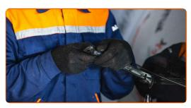
Remove the blade from the wiper arm.
