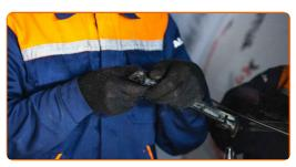
Remove the blade from the wiper arm.
