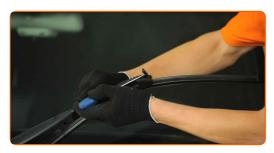
Remove the blade from the wiper arm.
