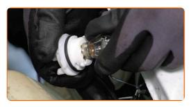
11 Remove the turn signal light bulb.
