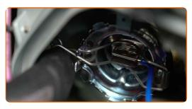
Attach the fog light bulb connector.
