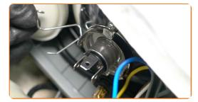
9 Remove the low and high beam bulb.
