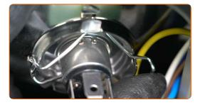
Attach the connector of the low and high beam bulb.
