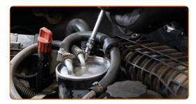
Detach the tubes from the fuel filter. Use round-nose pliers.
