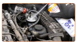
Loosen the fuel filter mounting. Use HEX No.H5. Use a ratchet wrench.
