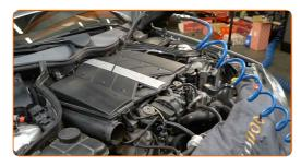
Remove the air filter housing.
