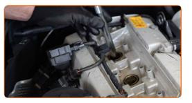
12 Screw new spark plugs and tighten them. Use the spark plug socket #16. Use a torque wrench. Tighten it to 28 nm torque.
