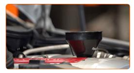
Screw the cap. Use the 76-14F socket. Use a torque wrench. Tighten it to 25 Nm torque.
