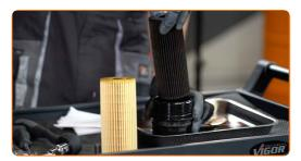
Replacement: engine oil and filter – MERCEDES-BENZ C-Class T-modell (\$203). Tip from AUTODOC experts:
