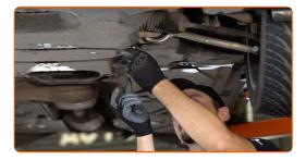
Undo the fasteners of the oil pan lower cover. Use a drive socket #8. Use a ratchet wrench.
