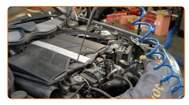
Remove the air filter housing.
