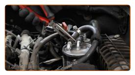
Replacement: fuel filter – MERCEDES-BENZ C-Class T-modell (S203). Tip:
