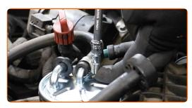
Press the fuel primer pump several times until it gets hard. Use a bulb hand fuel pump.
