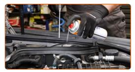
Attach the pipe to the fuel filter.
