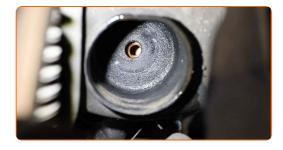
Screw in the lower fastener of the engine mount. Use a drive socket #16. Use a ratchet wrench.
