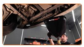
Unscrew the drain plug. Use a combination spanner #13.
