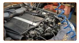
Remove the air filter housing.
