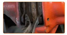
12 Remove the brake pads.
