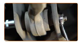
Unscrew the ball joint fastening to the steering knuckle. Use a combination spanner #21.
