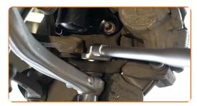
Tighten the fastener connecting the control arm to the subframe. Use a combination spanner #21. Use Torx E20. Use a torque wrench. Tighten it to 80 Nm torque.+120°
