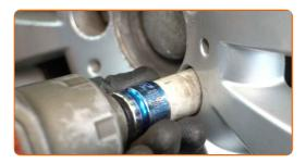
Lower the car and working in a cross order, tighten the wheel bolts. Use wheel impact socket #17. Use a torque wrench. Tighten it to 130 Nm torque.
